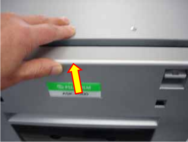
Fig.34 Close front door securely (until it becomes locked)
