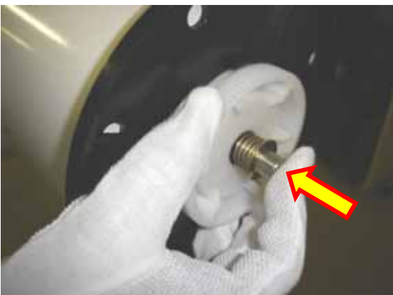
Fig.19 Left plate is locked if right plate shaft is pushed in
