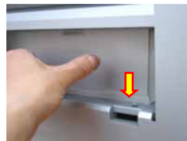
Fig.38 Fit protruded portion at the bottom of the slug box to the recessed part of slug box receptacle
