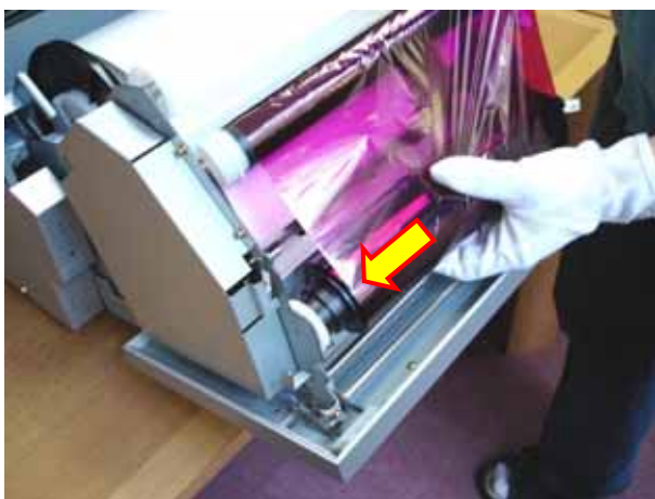
Fig.28 Push supply side bobbin with gear (black) to supply side ribbon gear
