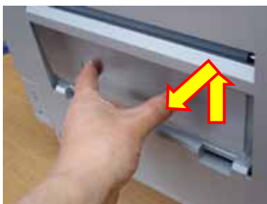
Fig.36 Lift up the slug box first and then pull it out
