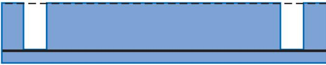
Figure 2b. Descender/Fill etch. Etch blind holes. This *Descender* will connect the pumping chamber to the nozzle. The *Fill* connects to fluid reservoir.
