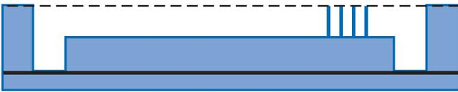
Figure 2c. Pumping Chamber/Filter Etch. Etch a rectangular pumping chamber with Acoustic Terminator at fill end.
