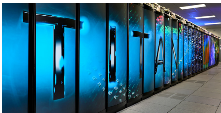
Oak Ridge National Labs is the home of the Titan supercomputer. Titan is a Cray XK7 system that contains 18,688 nodes, each built from a 16-core AMD Opteron 6274 processor and an NVIDIA Tesla K20X GPU accelerator. Titan also has 710 terabytes of memory.
