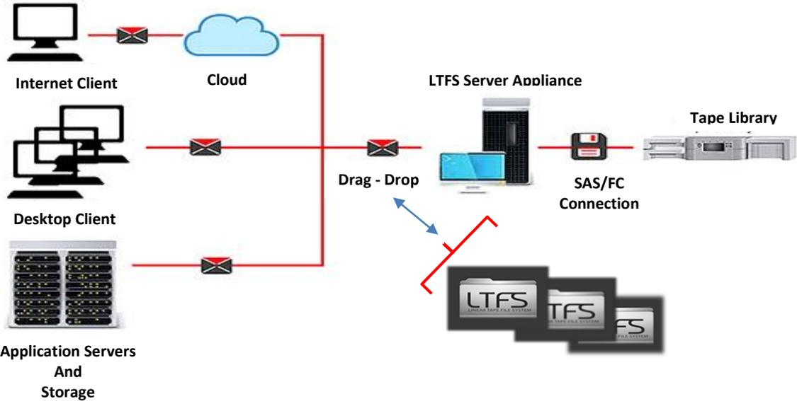
**Key point:** *LTFS is not a disk replacement but it changes the rules for tape access and enables much faster tape access than any previous tape format. With LTFS, tape looks and acts more like disk.*
