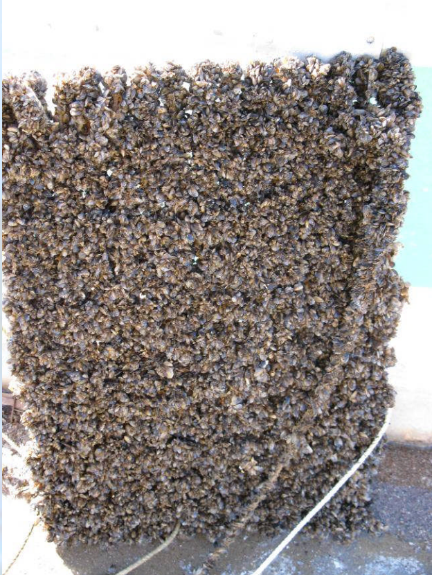
Un-coated Steel Grate – 8/08 through 12/08
