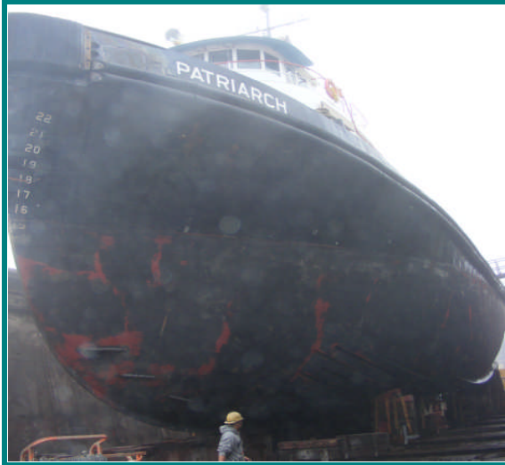
Prior to surface preparation and coatings
